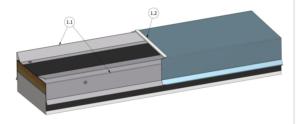
Step 1.1 Install Front and Back Cleats and secure with 10-9 x 1 1/8" ULP Fasteners.
